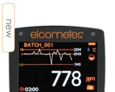
On-screen run graph shows last 20 measurement values
