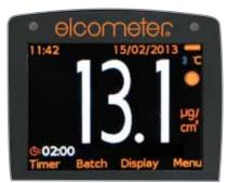
Large colour LCD screen displays readings in  $\mu g/cm^2$ , ppm,  $\mu S/cm$ , mS/cm, % salinity or mg/m<sup>2</sup>
