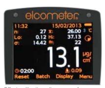
Offset calibration allows use of non-pure water
